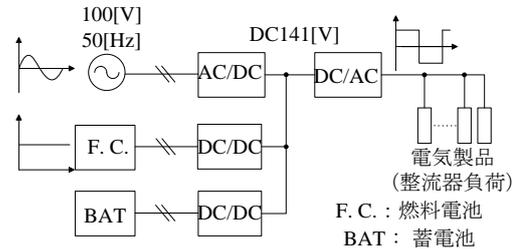
Fig. 1. Proposed system of square-wave distribution applied to smart house
