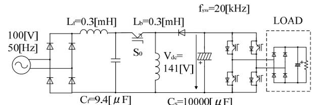
Fig. 3. Circuit of single phase buck/boost PFC converter
