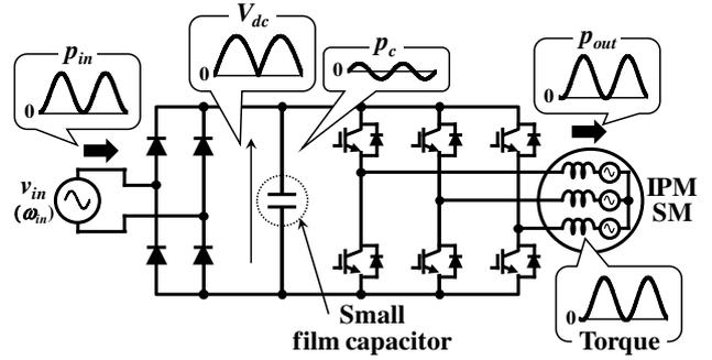
Fig. 2. Electrolytic capacitor-less single inverter.
