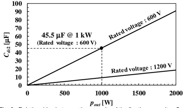
Fig. 8. Relationships between the capacity of the floating capacitor  $C_{dc2}$ , the output power  $p_{out}$  and the rated voltage of INV2.
