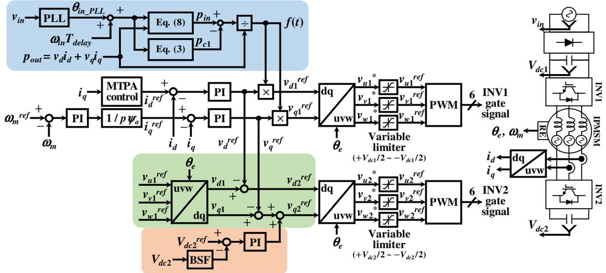
Fig. 9. Proposed block diagram based on the high input power factor control method, suppression control method of torque pulsation and input capacitor voltage control method of floating inverter.
