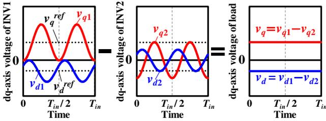
Fig. 6. Relationship between the output dq-axis voltages of each inverter and the load dq-axis voltage.
