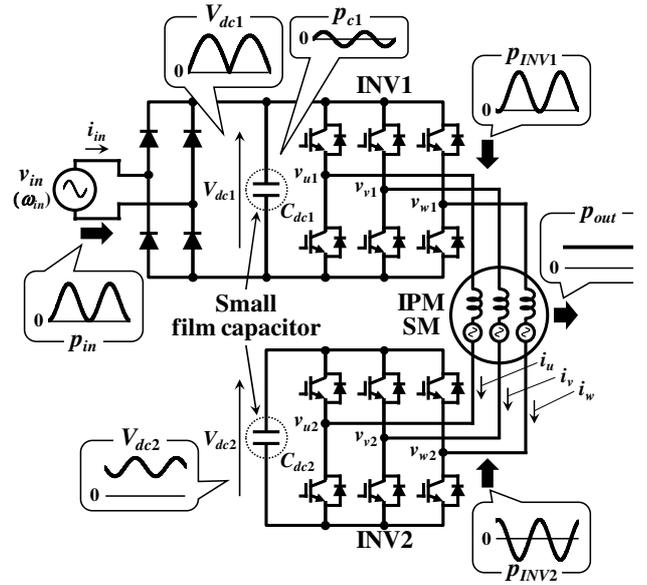
Fig. 3. Electrolytic capacitor-less dual inverter.
