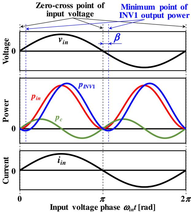
Fig. 5. Relationship between each power and single-phase ac voltage.
