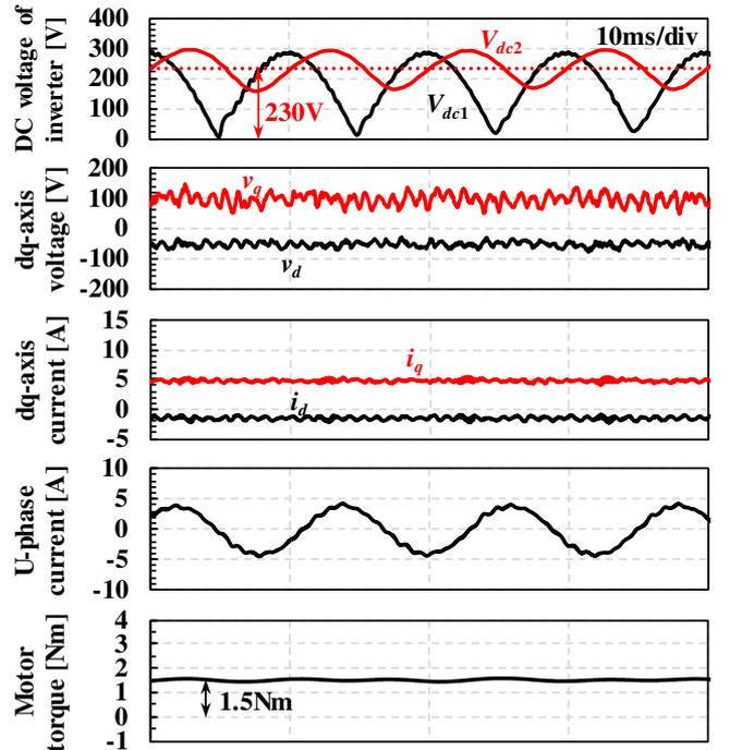
Fig. 12. Experimental results of the proposed electrolytic capacitor-less dual inverter at 2500 rpm and 1.5 Nm. From top to bottom, the dc voltage of INV1 and INV2, load dq-axis voltage, dq-axis current, U-phase current, and load motor torque.
