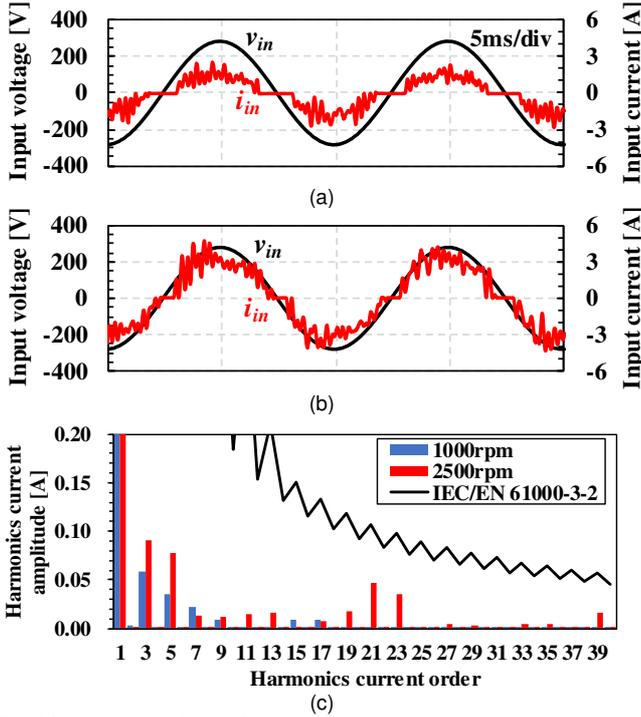
Fig. 14. Input waveform of the electrolytic capacitor-less dual inverter. (a) 1000 rpm. (b) 2500 rpm. (c) FFT analysis results of input current at each speed.
