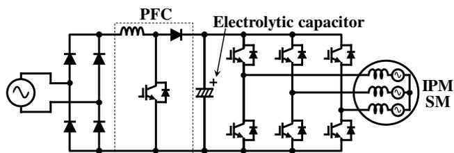
Fig. 1. Single inverter with unidirectional boost type PFC and an electrolytic capacitor.
