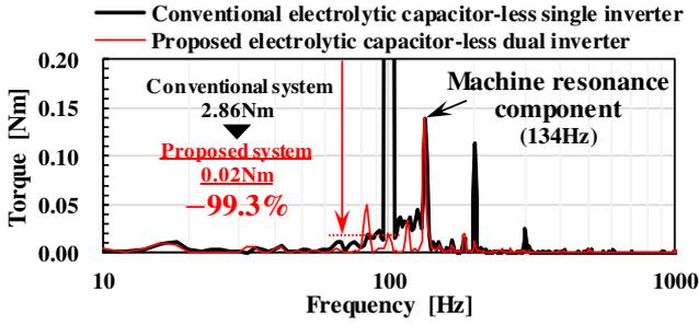
Fig. 13. FFT analysis results of motor torque in the proposed system.
