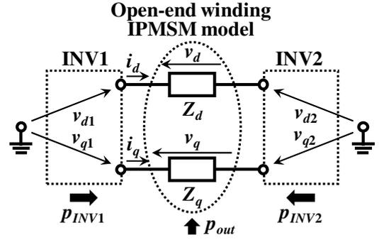
Fig. 4. Dual inverter power, dq-axis voltage and dq-axis current.
