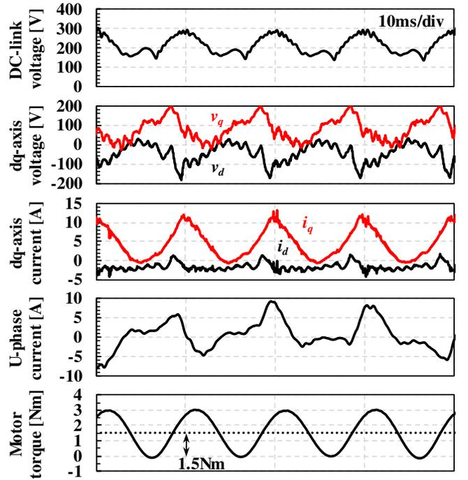
Fig. 11. Experimental results of the conventional electrolytic capacitor-less single inverter at 2500 rpm and 1.5 Nm. From top to bottom, the dc-link voltage, load dq-axis voltage, dq-axis current, U-phase current, and load motor torque.
