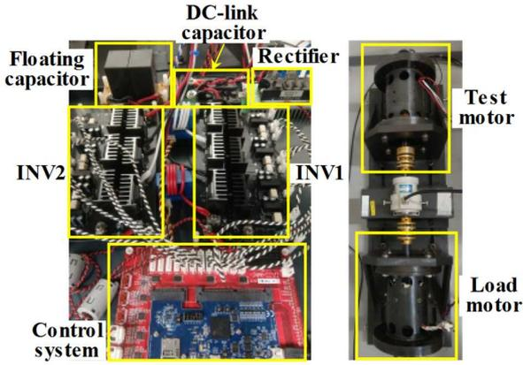
Fig. 10. Experimental setup.
