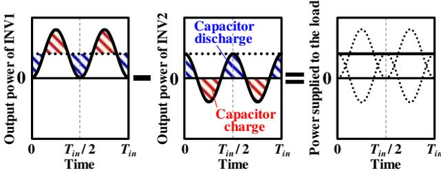
Fig. 7. Relationship between the output powers of each inverter, the load power and the state of capacitor charge or discharge.
