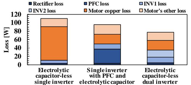
Fig. 16. Loss breakdown of the electrolytic capacitor-less single inverter, single inverter with PFC and electrolytic capacitor and electrolytic capacitor-less dual inverter.
