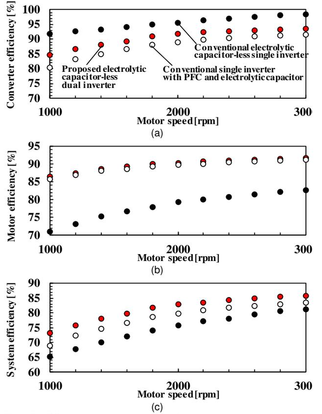
Fig. 15. Efficiency analysis results of the conventional electrolytic capacitor-less single inverter, conventional single inverter with PFC and electrolytic capacitor, and proposed electrolytic capacitor-less dual inverter at 1.5 Nm. (a) Converter efficiency. (b) Motor efficiency. (c) System efficiency.
