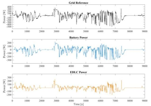
Fig. 18: 1:3 power ratio experiment. Grid power reference, battery power reference and EDLC power reference
