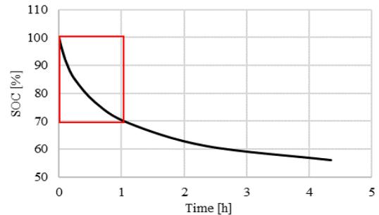
Fig. 7: EDLC self-discharge trend in a 4-hour period from 100% SOC.
