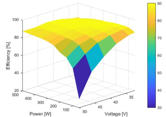
Fig. 11: EDLC pack and EDLC side DC/DC converter combined efficiency at 33 V to 50 V (39% SOC to 95% SOC).
