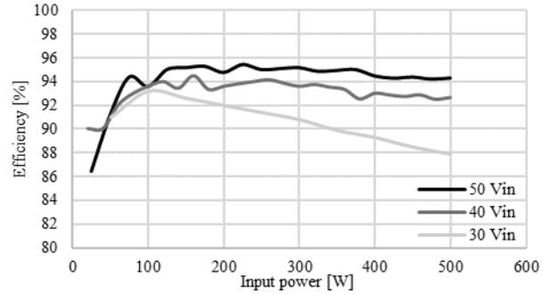
Fig. 8: Converter boost mode efficiency at 30, 40 and 50 Vin, 120
