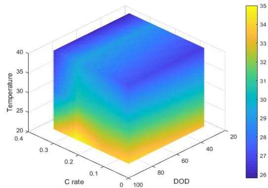
Fig. 5: Battery ESR relation with temperature, C rate and DOD.
