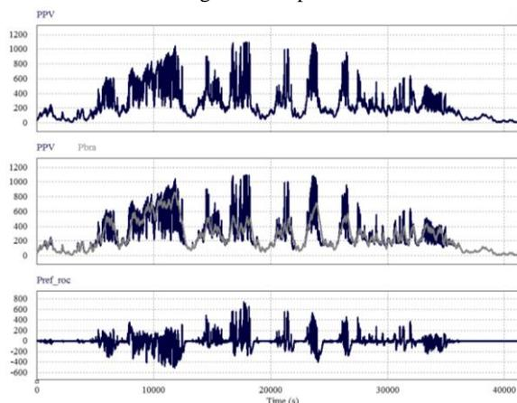
Fig. 2: PV power generation, filtered power and power to be attenuated
