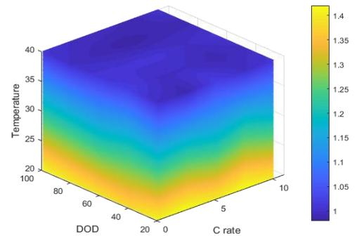
Fig. 6: EDLC ESR relation with temperature, C rate and DOD.
