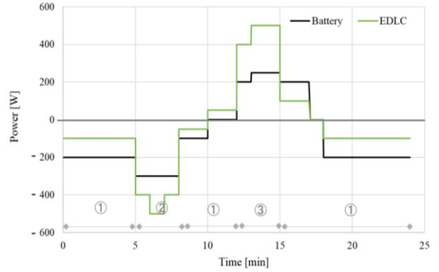
Fig. 12: ATBM example battery power reference and EDLC power reference
