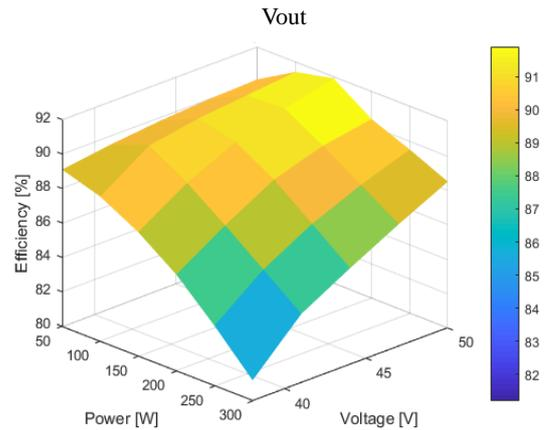
Fig. 10: Battery pack and battery side DC/DC converter combined efficiency at 38 V to 50 V (10% SOC to 95% SOC).
