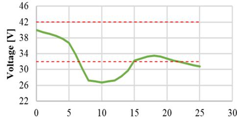
Fig. 14: ATBM example EDLC voltage trend
