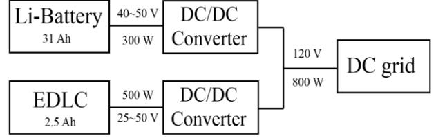
Fig. 16: Experimental system configuration schematic
