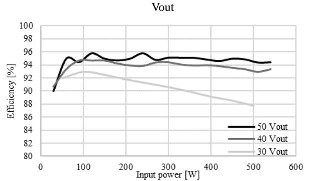
Fig. 9: Converter buck mode efficiency at 30, 40 and 50 Vin, 120
