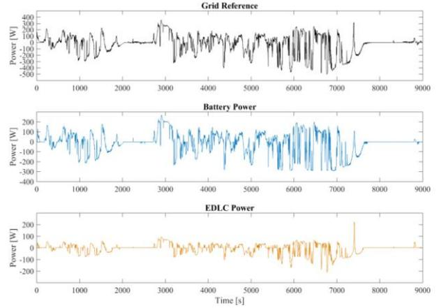
Fig. 17: 1:4 power ratio experiment. Grid power reference, battery power reference and EDLC power reference
