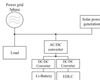
Fig. 1: Stabilization system connected to the grid and PV generation plant
