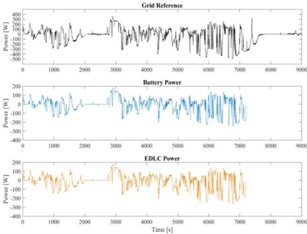
Fig. 19: 1:4 power ratio experiment. Grid power reference, battery power reference and EDLC power reference
