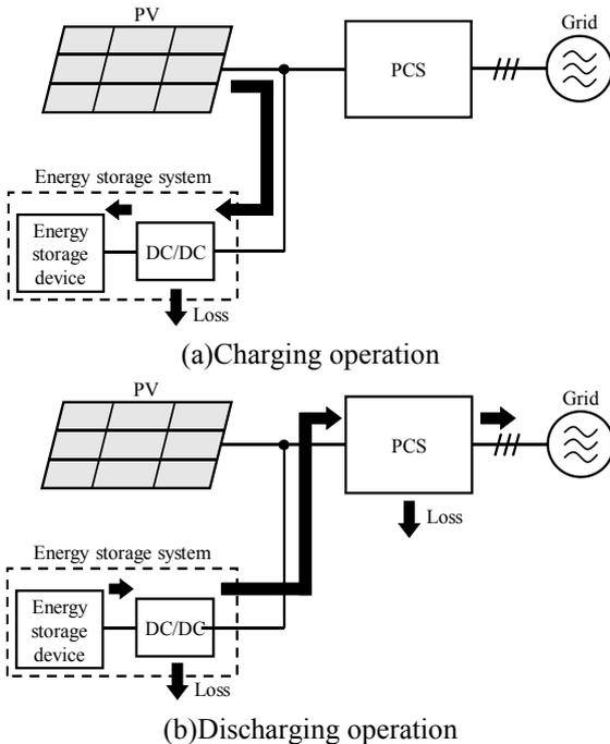
Fig. 4. Energy flow during charging and discharging of the energy storage system.
