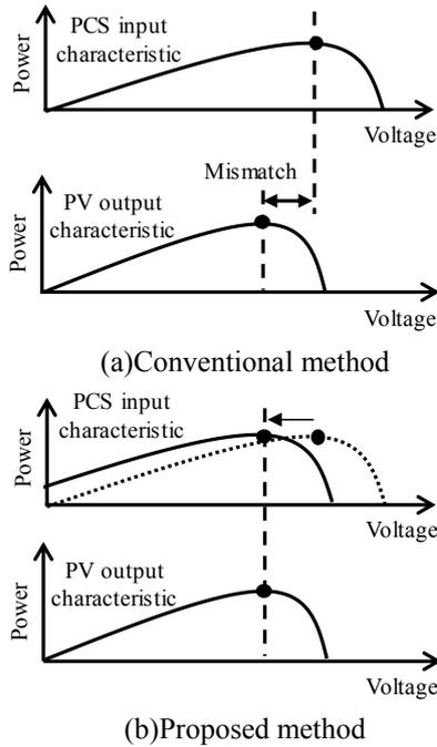
Fig. 6. Power characteristics at discharging operation.
