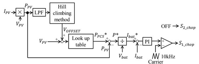
Fig. 8. Control block in discharging.
