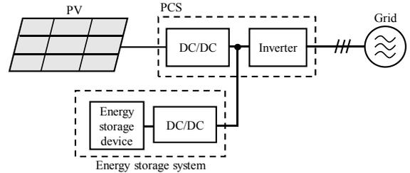
(b) Connection between DC/DC converter and inverter
