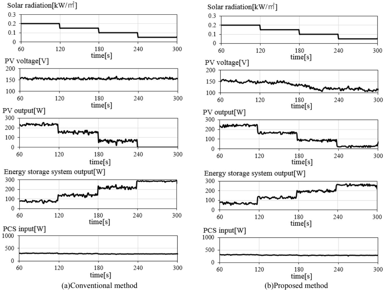
Fig. 10. Experimental results in discharging.
