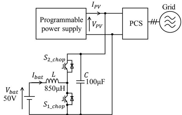
Fig. 7. Experimental structure.
