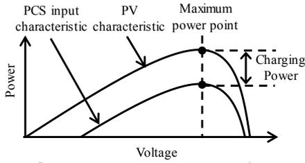
Fig. 5. Power characteristics at charging operation.
