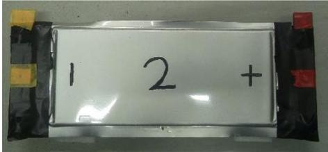
Fig. 5. Single 3.6 V Li-ion cell used in the battery pack
