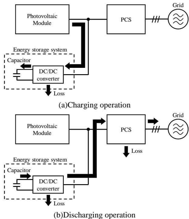
Fig. 12. Energy flow during charging and discharging of the energy storage system.
