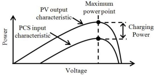
Fig. 5. Power characteristic of charging power.
