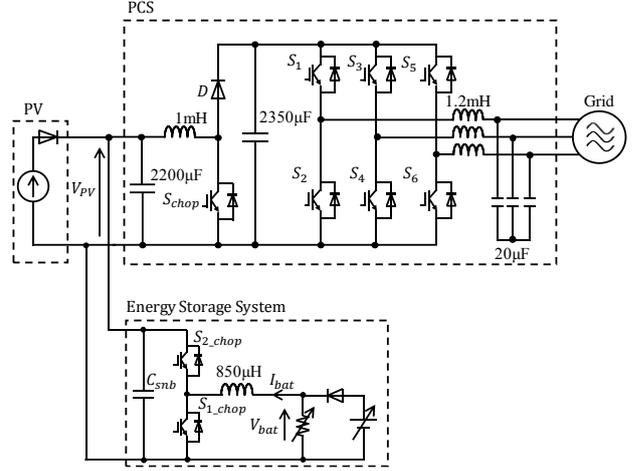
Fig. 6. Experimental structure.
