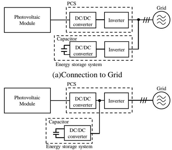
Fig. 2. Connection points of energy storage system.
