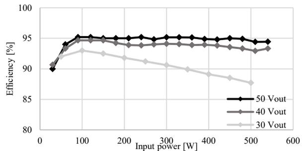
(a) Buck mode efficiency at 30, 40 and 50 Vout, 120 V input.
