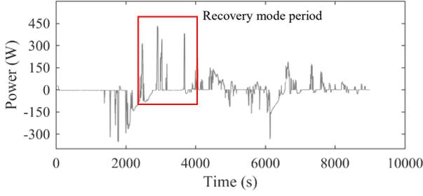
Fig. 17. ATBM experiment EDLC pack power reference after applying ATBM division method.
