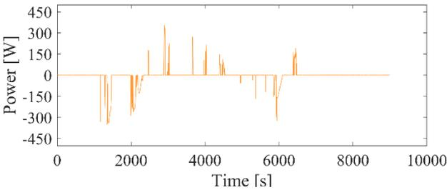
Fig. 20. ADAM experiment EDLC pack power reference after applying ADAM division method.
