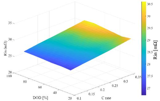
Fig. 3. Battery ESR relation with C rate and DOD.
