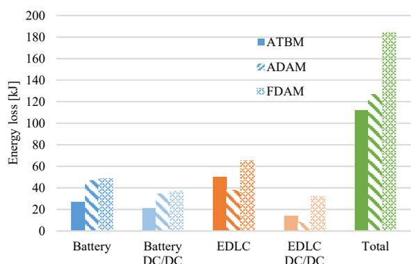
Fig. 23. Experimental ADAM and ATBM energy loss performance comparison.
