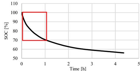
Fig. 5. EDLC self-discharge trend in a 4-hour period.
