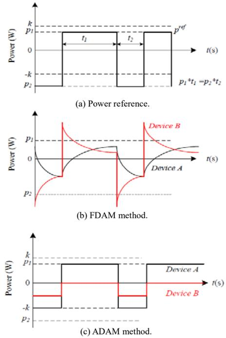
Fig. 2 Conventional methods of power division example.
