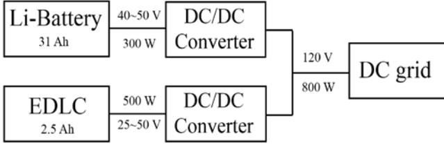
Fig. 6. Fluctuation balancing system schematic.
