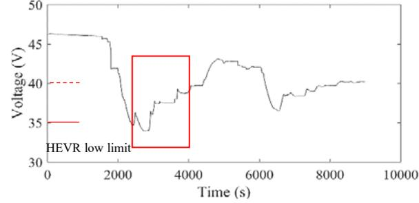
Fig. 18. ATBM experiment EDLC pack voltage response with recovery mode effect and threshold.
