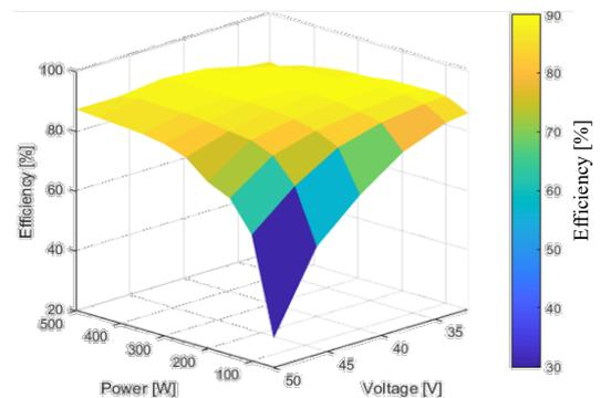
(b) EDLC pack and EDLC side converter combined efficiency at 33 V to 50 V (39% SOC to 95% SOC).
