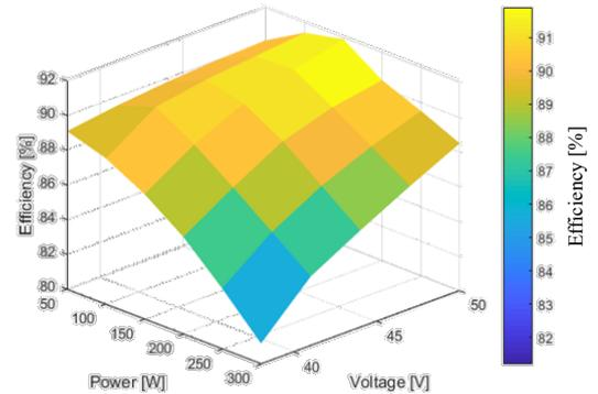
(a) Battery pack and battery side converter combined efficiency at 38 V to 50 V (10% SOC to 95% SOC).
