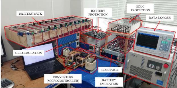
Fig. 14. Power fluctuation experimental prototype front view
