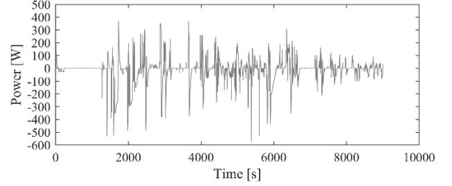
Fig. 22. FDAM experiment EDLC pack power reference after applying FDAM division method.
