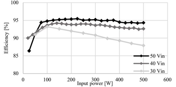
(a) Boost mode efficiency at 30, 40 and 50 Vin, 120 V output.
