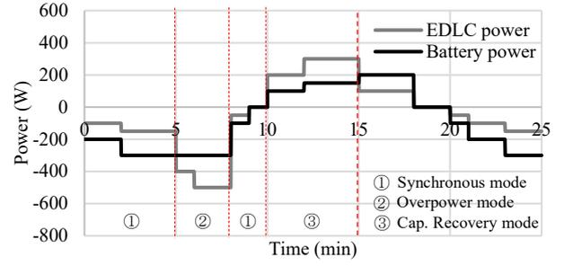
Fig. 9. Proposed method ATBM (Active Threshold Balancing Method) example power division example.
