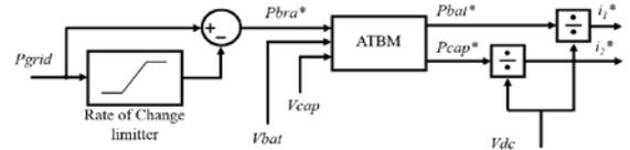
Fig. 12. Experimental proposed control block diagram
