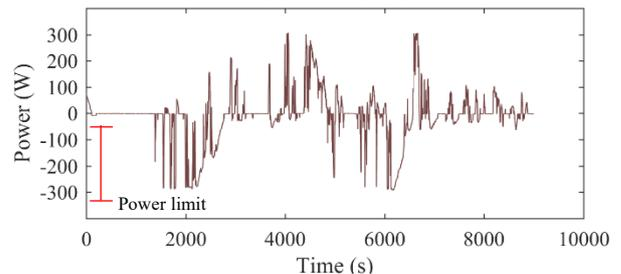
Fig. 16. ATBM experiment battery pack power reference after applying ATBM division method.
